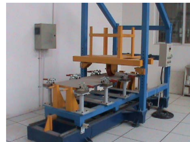
滚动荷载检测设备 Rolling Capacity Tester
