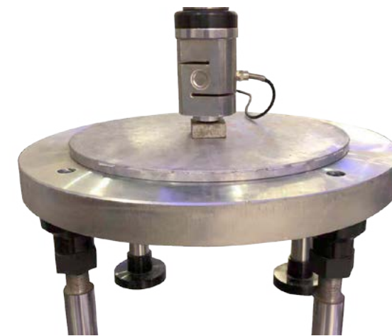
铝盖板检测设备(电脑曲线图) Aluminium Alloy Circular Panel Loading Capacity Tester
